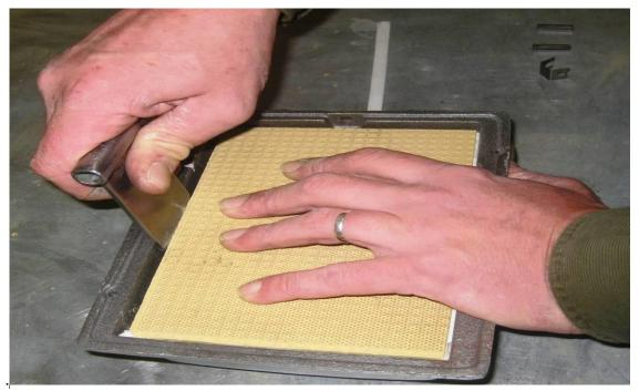
6. Press with the help of a tool the stone against the frame list creating a space for the last frame list and hold it in position with the other hand.
