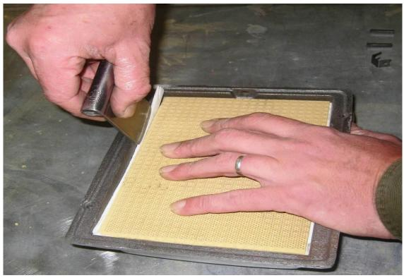
7. Press gently with the help of a tool the last frame list in its position.
