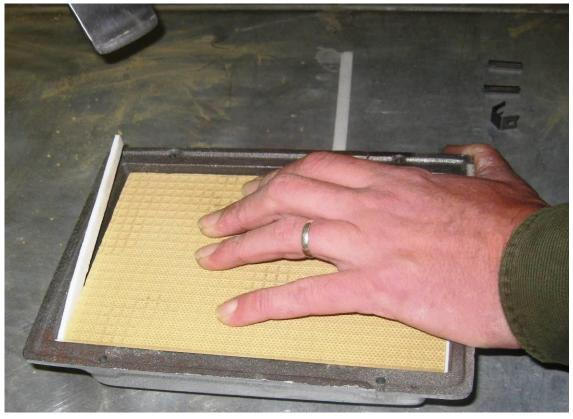
5. Place the frame list in the short side position and press it gently in the gap next to the stone and the housing with a steel or wooden tool. Take care of not damaging the stone.
